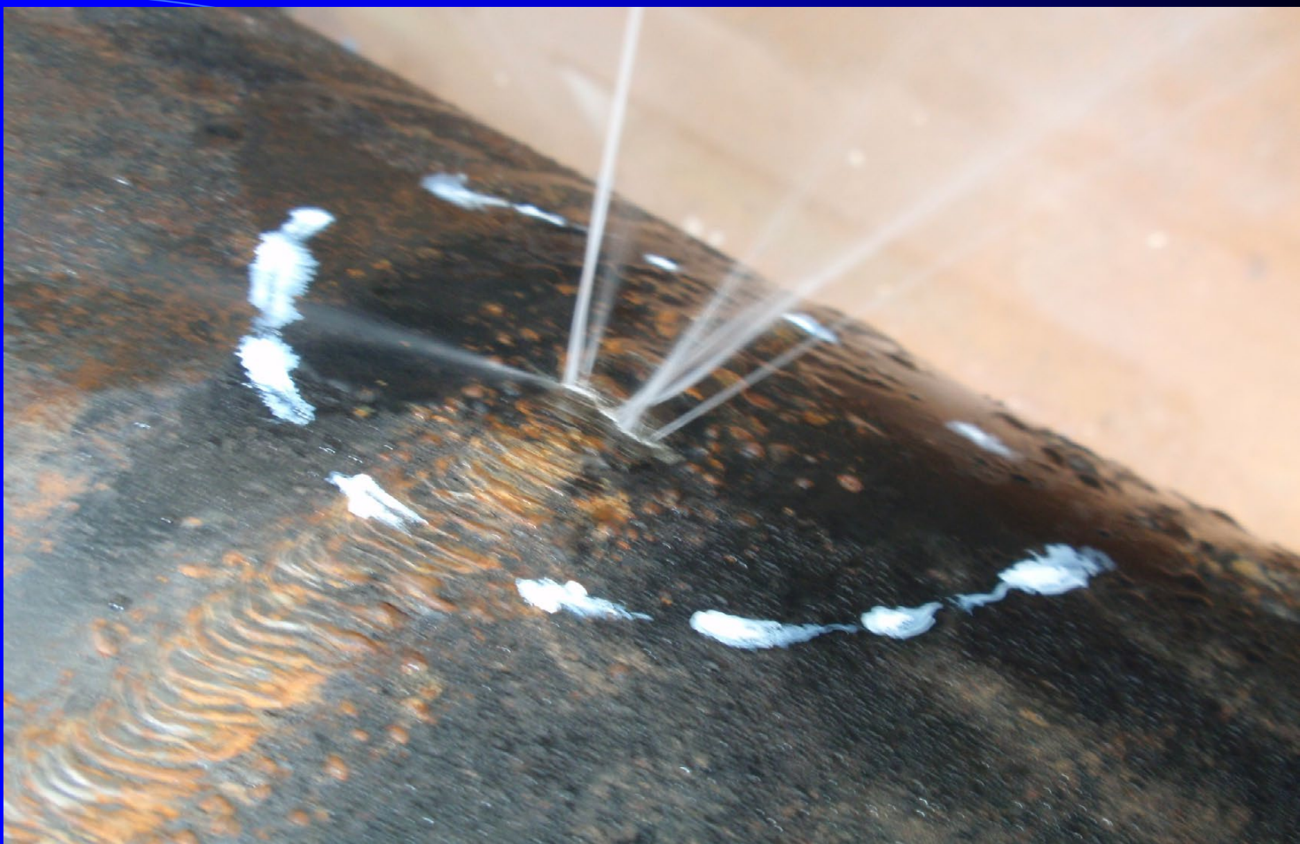
Destruction of circumferential weld
