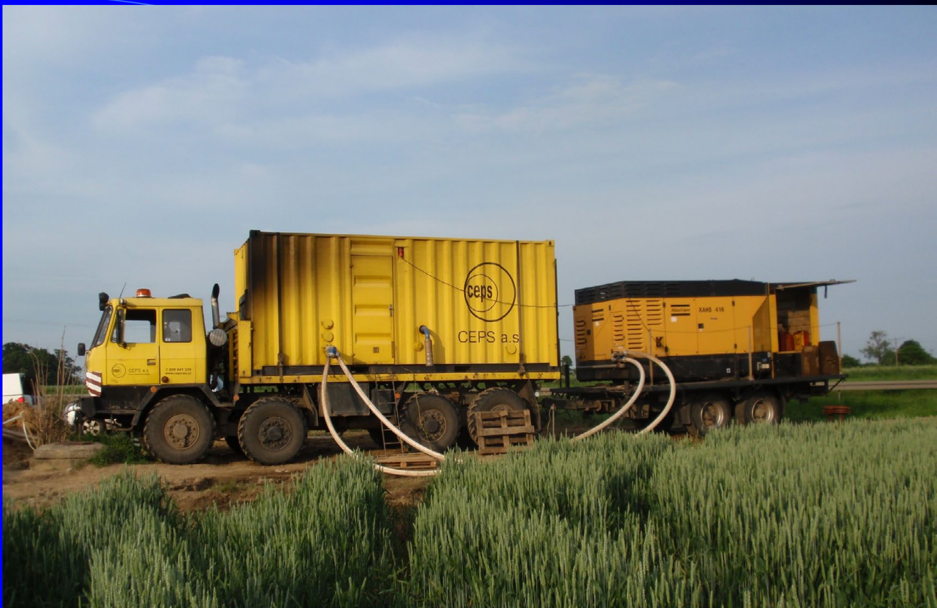
The mobile drying unit
