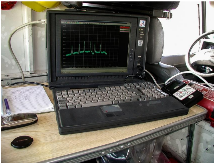
The record of six hydrogen traces at the end of measured part of DN 1400 gas pipeline with length of 50 km. The traces were injected into the gas flow in the intervals of several minutes.
