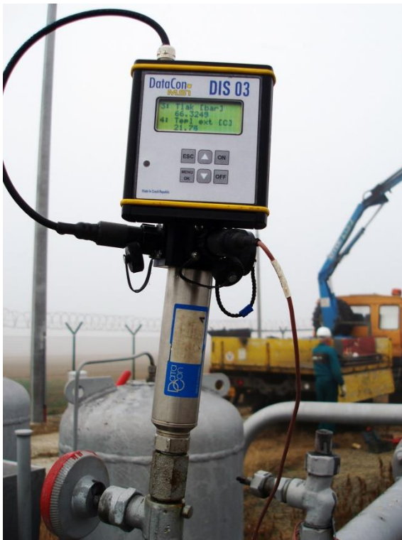
High-precise gauge/recorder of pressure and temperature
