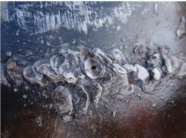
A flawed circumferential weld in the field burst under testing. A close-up shows both the lack of workmanship in the initial weld and the defect which failed (Figs. 4 and 5).
