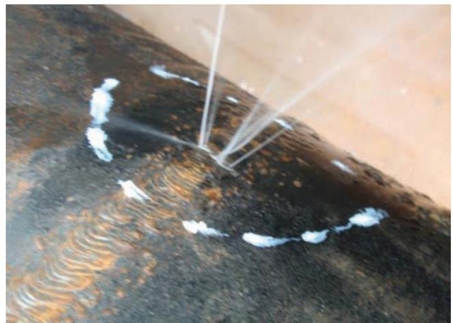
The pipe body vessel was destroyed on the circumferential weld at 16,632 MPa (Figs. 1 and 2).
