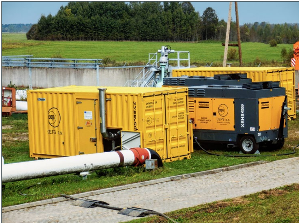
Figure 9: Production of nitrogen mixture on the jobsite
